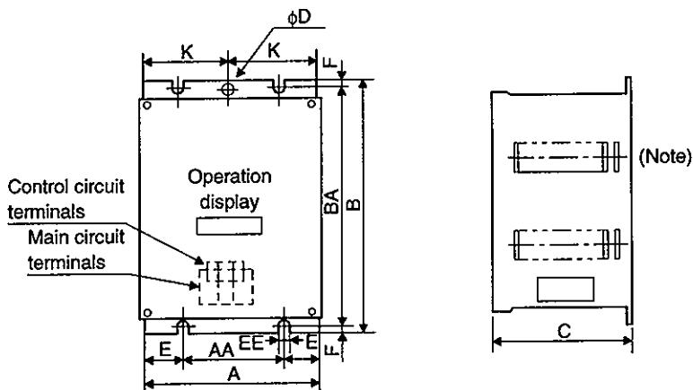
Note: Ventilation ports are provided in both side faces and top face. The bottom face is open.
