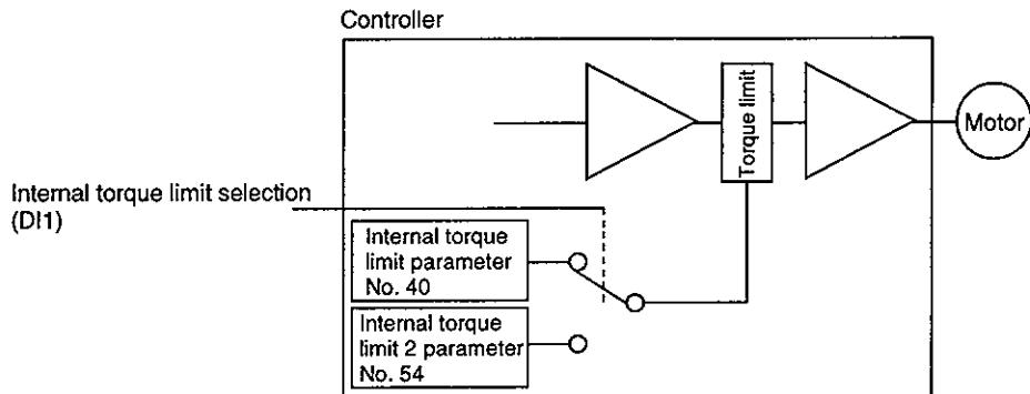
Using the internal torque limit selection (DI1), choose the limit value as follows. When DI1-SG are shorted, the smaller value of the internal torque limit and internal torque limit 2 is chosen:
