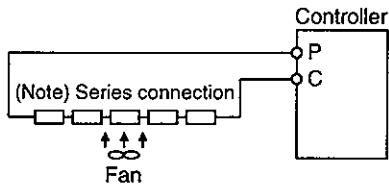
Note: The number of resistors connected in series depends on the resistor type.
