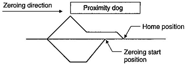
At a start, a motion is made in the zeroing direction and an automatic return is made on detection of the limit switch. The motion stops past the front end of the proximity dog, and zeroing is resumed at that position. If the proximity dog cannot be detected, the motion stops on detection of the opposite limit switch and AL 90 occurs.
