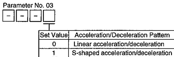
For linear acceleration/deceleration pattern, to select the liner acceleration/deceleration pattern, set □□0 in parameter No.3.
