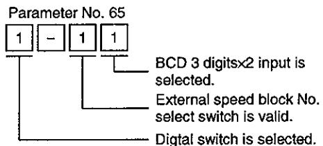
Using the digital switch (MR-DS60), set the position data (increment). The unit ([mm], [[inch]) and input range of the position data (increment) can be changed by setting parameter No.4.
