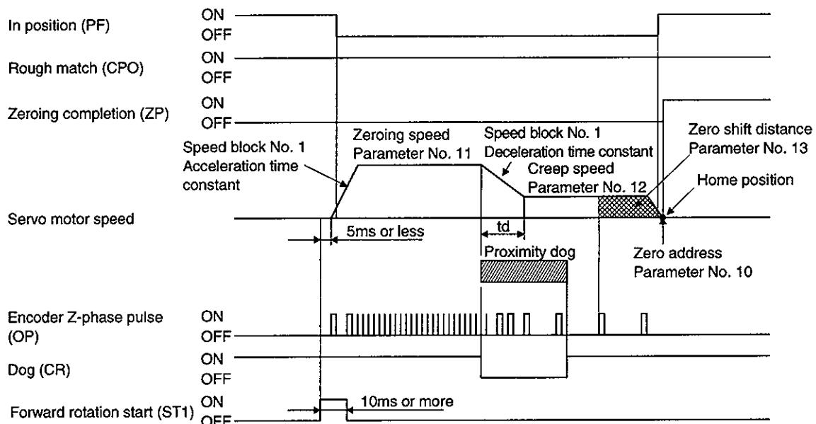
The address on completion of zeroing is the value automatically set in parameter No.10 (zeroing position data).
