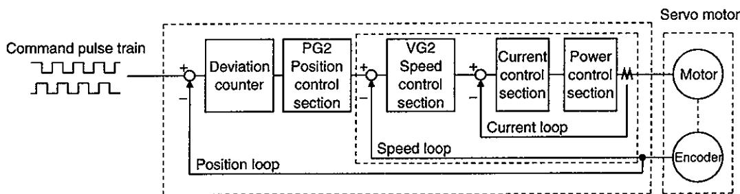
A general servo system configuration is shown above. The servo control system consists of three loops: current loop, speed loop and position loop. Among these three loops, the response of the inside loop must be increased 4 to 6 times higher. If this condition is not satisfied, vibration will be generated. If the condition further worsens, hunting will occur.
