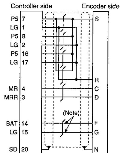
Note: This wiring is required for use in the absolute position detection system.
