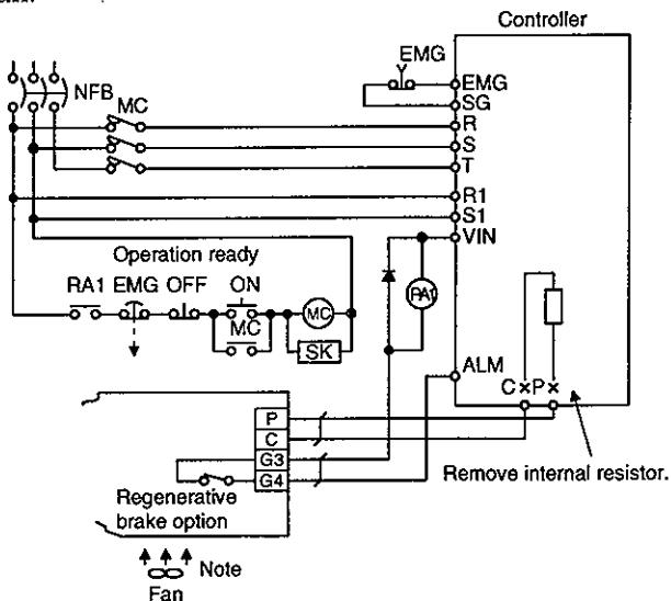
Note: When the MR-RB5□ is used, cool it forcibly by the cooling fan ( $1.0\text{m}^2/\text{min}$ , about □92).
