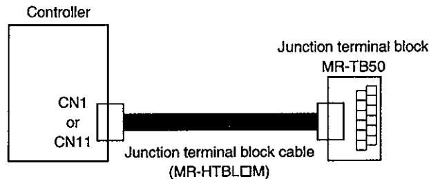
Ground the junction terminal block cable on the junction terminal block side with the standard accessory cable clamp fitting (AERSBAN-ESET). For the use of the cable clamp fitting, refer to (3), Section 15.2.6
