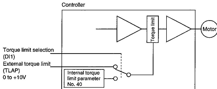
Using the internal torque limit selection (DI1), choose the limit value as follows. When DI1-SG are shorted, the smaller value of the external torque limit and internal torque limit is chosen:
