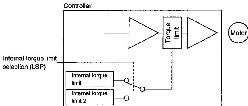
Using the internal torque limit selection (LSD), choose the limit value as follows. When LSD-SG are shorted, the smaller value of the internal torque limit and internal torque limit 2 is chosen:
