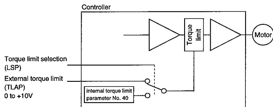
Using the internal torque limit selection (LSP), choose the limit value as follows. When LSD-SG are shorted, the smaller value of the external torque limit and internal torque limit is chosen:
