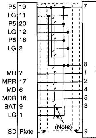
Note: This wiring is required for use in the absolute position detection system.
