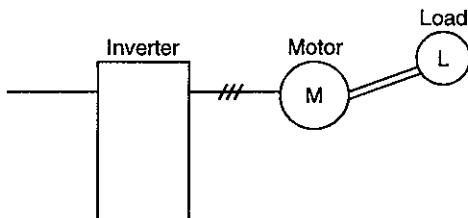
On the other hand, the servo amplifier always detects the positions and speeds of the motor and machine using the servo motor encoder, and exercises control to match the position and speed commands with the actual motor (machine) position and speed. In the servo system, adjustment is needed because:
