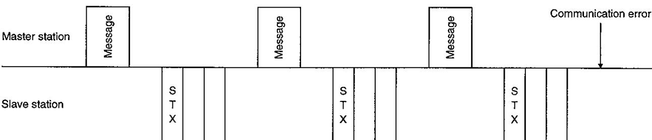
Similarly, when the master station detects a fault (e.g. checksum, parity) in the response data from the slave station, the master station retransmits the message which was sent at the occurrence of the fault. A communication error occurs if the retry operation is performed three times.
