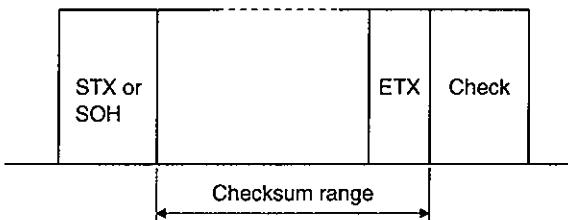
The checksum is sent as a JIS8-coded hexadecimal code representing the lower two digits of the sum of JIS8-coded hexadecimal values up to ETX, with the exception of the first control code (STX or SOH).
