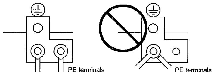
2. For the grounding of the control box, refer to EN60204.
