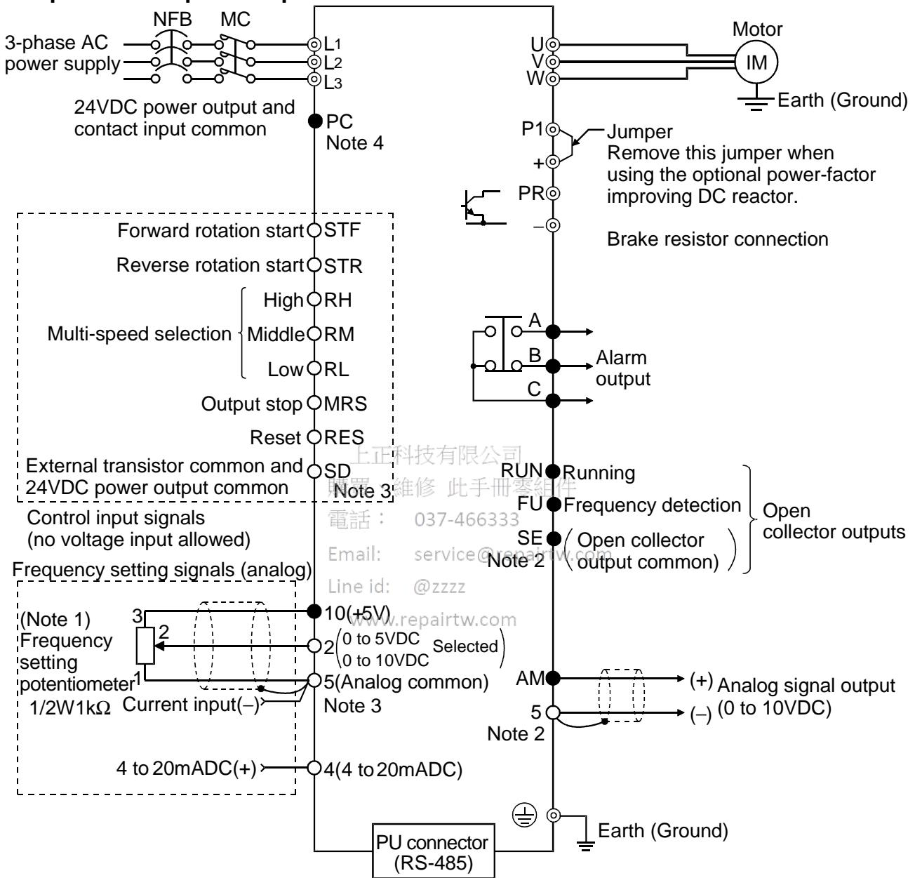
Note: 1. If the potentiometer is to be operated often, use a 2W1kΩ potentiometer.
